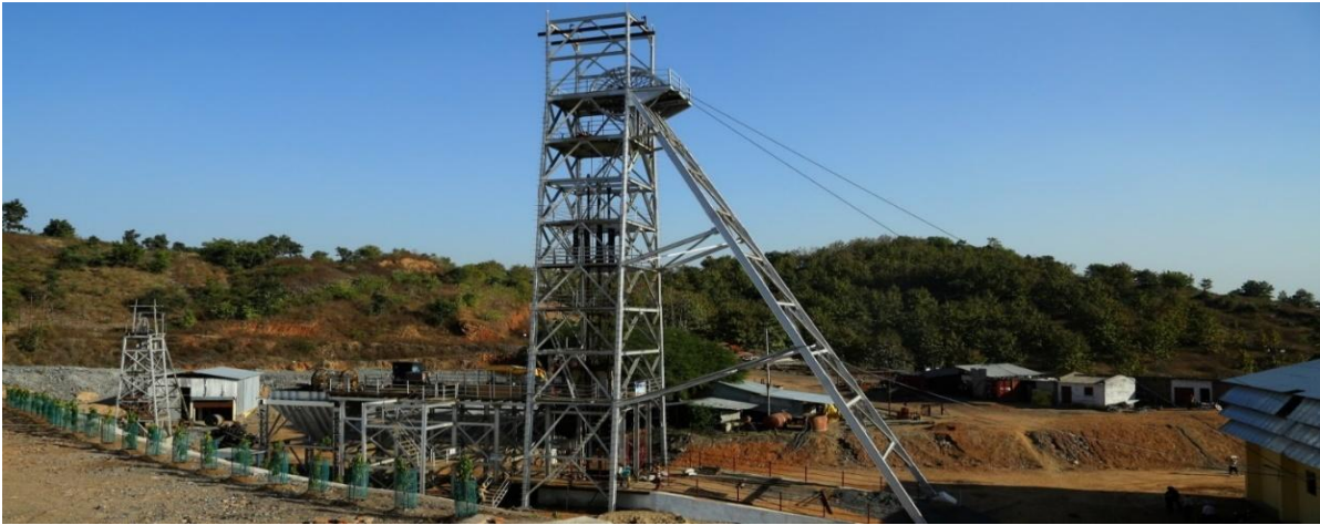
Figure 40: Sinking of vertical shafts at Munsar Mine & Ukwa Mine of MOIL Limited
